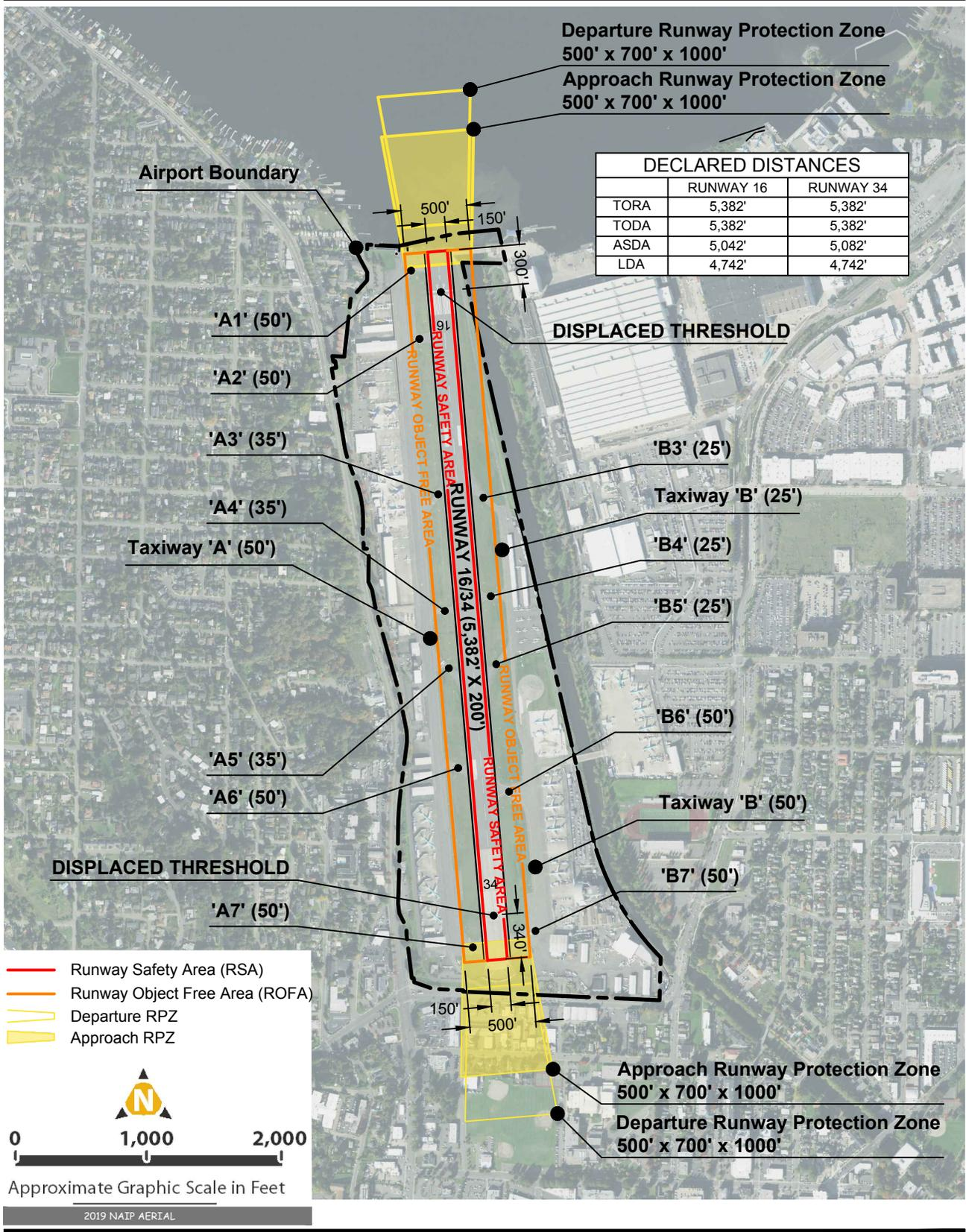
FIGURE B1 Existing RDC B-II Design Standards
